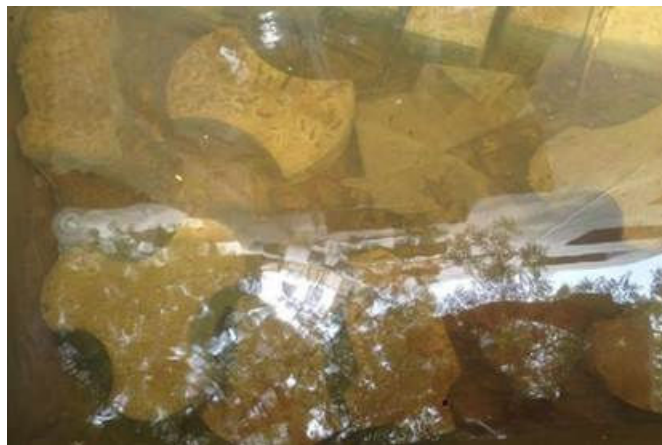
Figure 2.3: Curing process for paver blocks
