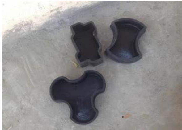
Figure 2.1: Different shapes of paver moulds
