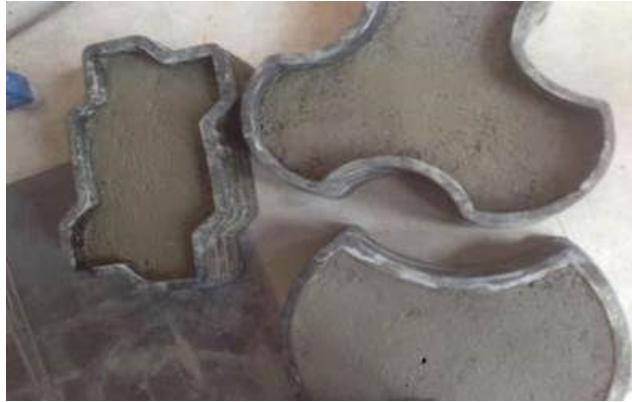
Figure 2.2: Paver blocks after being moulded
